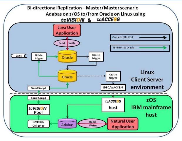
This is a simplified representation of the replication scenario between the z/OS mainframe with ADABAS and the LINUX platform with ORACLE.
